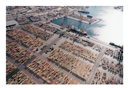
Pier I in particular is trapezoid shape and is aligned in the North/South direction, positioned at the eastern side of the Container Terminal. The total length of the dock is 763 meters, of which 300 meters on the eastern side, 178 meters on the southern front and 285 meters on the western side. The net depth by the western dock (where rail-tracks for the operation of the gantry cranes have been installed) is 12 meters.
